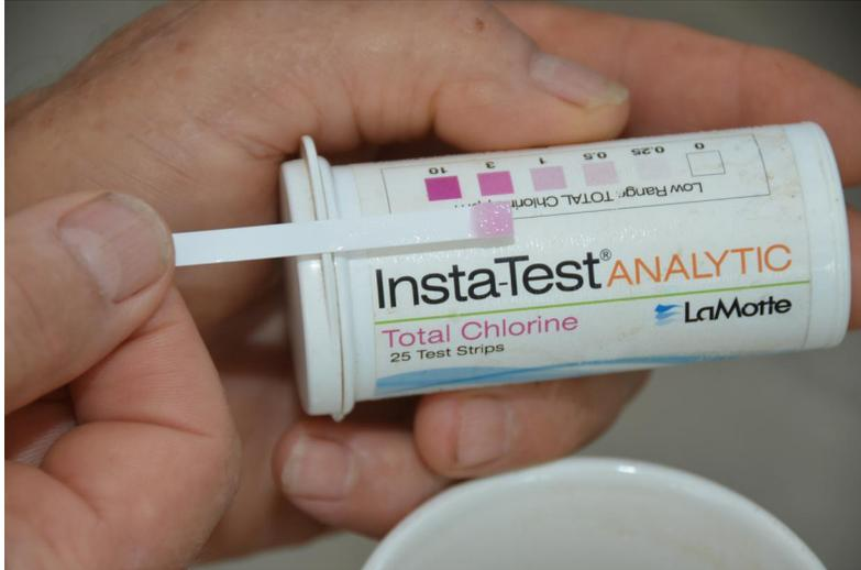
**Ammonia and nitrite/nitrate test strips work just like these chlorine test strips: you dip them into the water, then compare the color on the pad to the color on the bottle to get your reading.**
