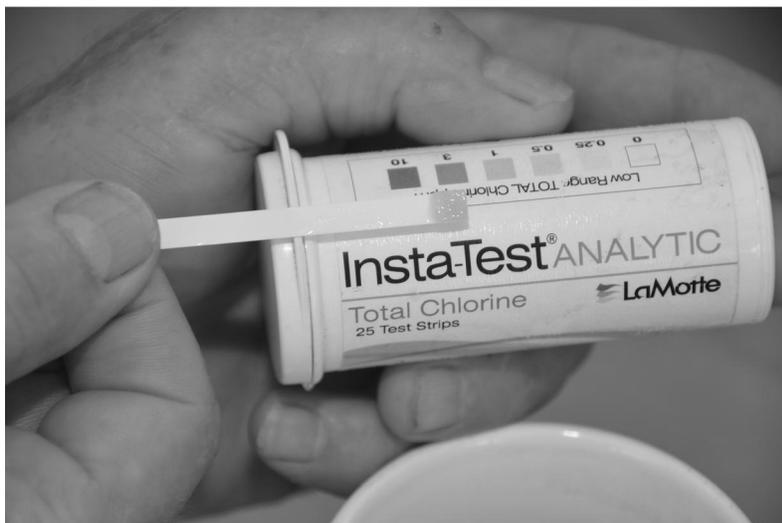
**"Total" Chlorine test strips test for both chlorine and chloramines in your incoming water.**
